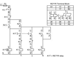
⚠ No galvanic insulation between supply terminals A1, A2, B1, B2 and control input Z2. This terminal must therefore never be used (factory setting).
